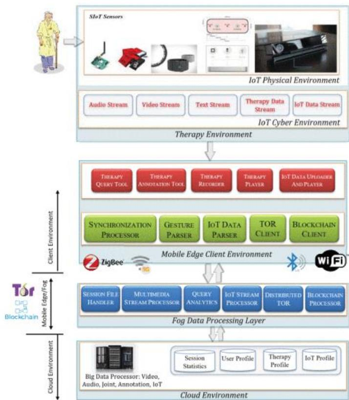
**Figure 18.** Secure data flow of MEC therapy application through different environments (Rahman et al., 2018)
