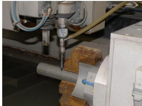
**Figure 3.** WPC sample in the clamps – AWJ/WJ turning (HutYROVA et al., 2016)
