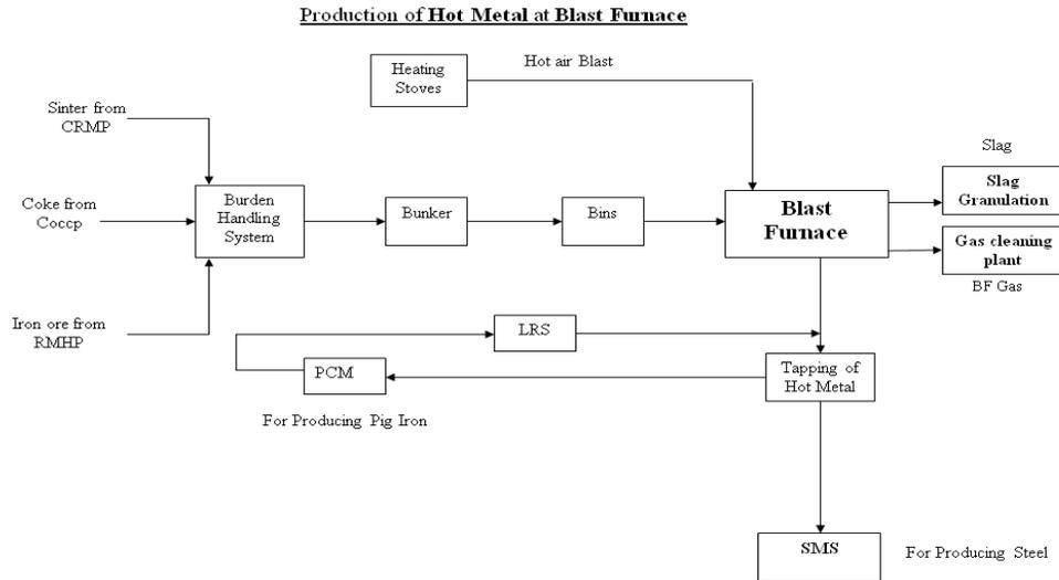
**Figure 1.** Process flow diagram of Hot Metal process in Blast Furnace
