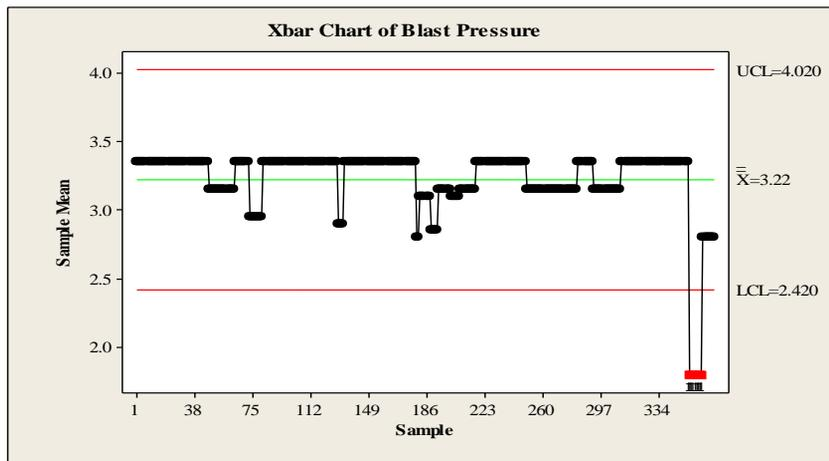
Figure 2.  $\bar{X}$ Chart of Blast Pressure
