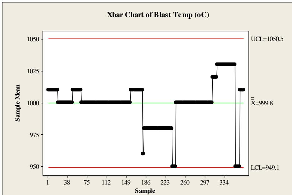
**Figure 4.**  $\bar{X}$ Chart of Blast Temperature
