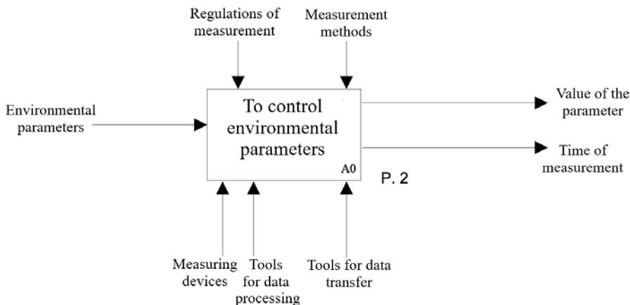
**Figure 8.** Initial consolidated context diagram A-0 of functional logical and informational model of PCS
