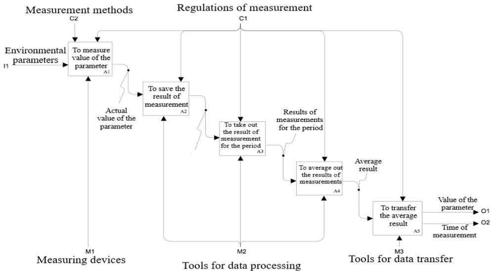
**Figure 9.** Decomposition of the first level of A-0 functional logical and informational model of PCS business processes
