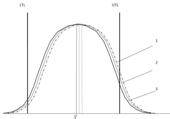
**Figure 2.** Gauss curves describing a production process 1, 2, 3 are production process states
