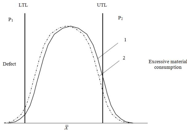
Figure 4. Change of a production process state with time 1, 2 are production process states
