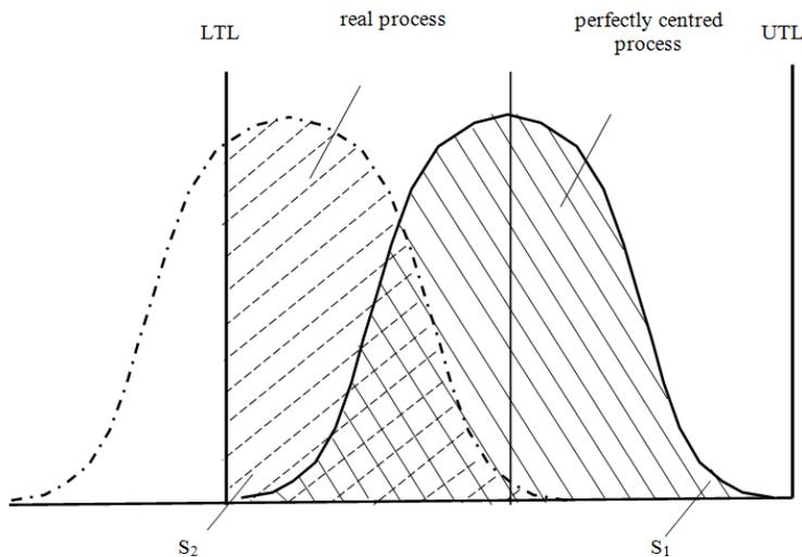
Figure 8. Method of Qp index calculation
