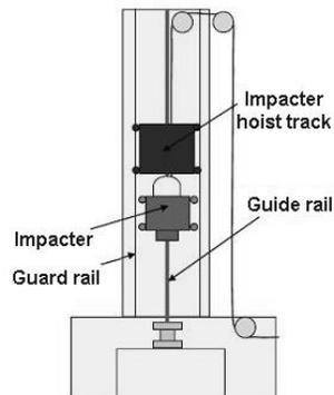
Figure 13. Drop-weight test equipment
