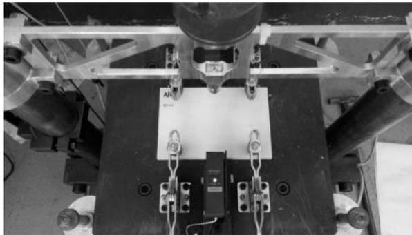
**Figure 14.** Drop-weight test of Grès Porcelain tiles
