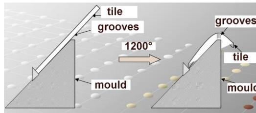
Figure 4. Bending process
