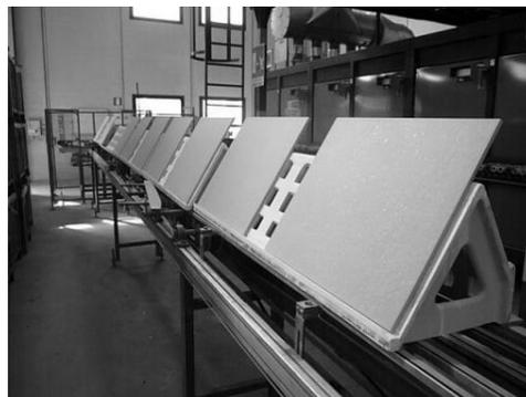
Figure 5. Tiles before bending process
