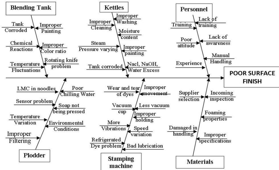
*Fig 5 Cause and effect diagram for poor surface finish*
