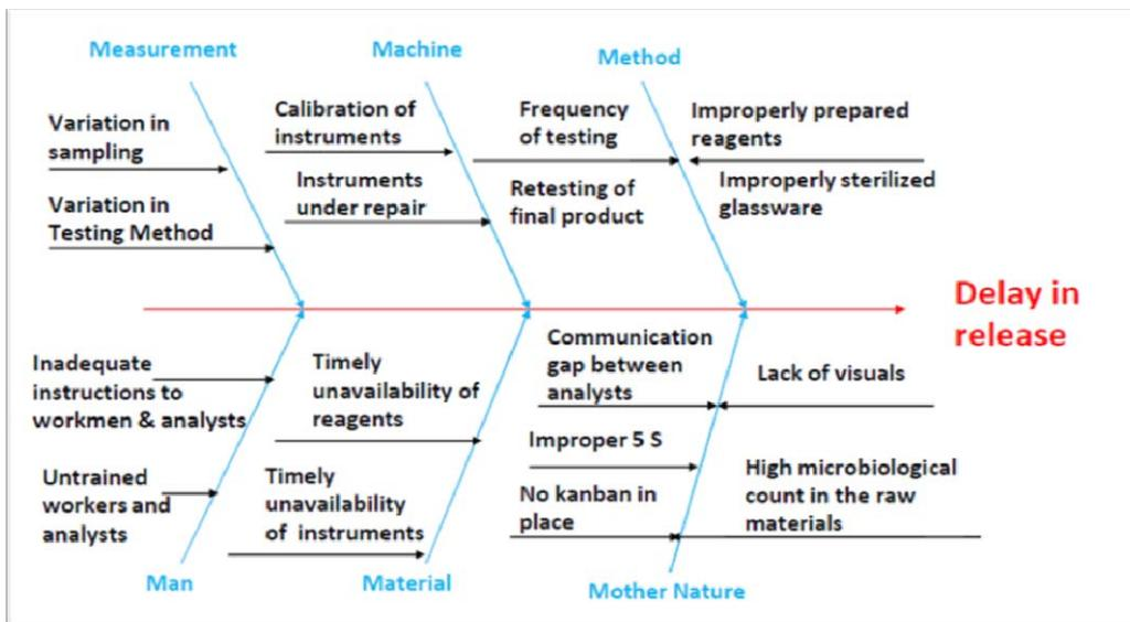
Figure 1 Fishbone diagram: Cause and effect
