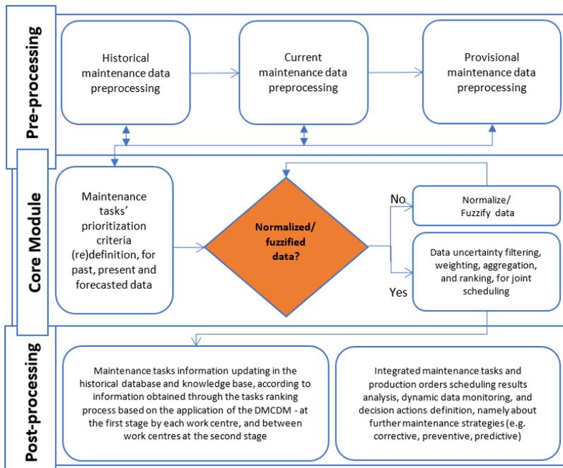
Figure 3. Proposed maintenance tasks processing methodology based on a two-stage assessment method
