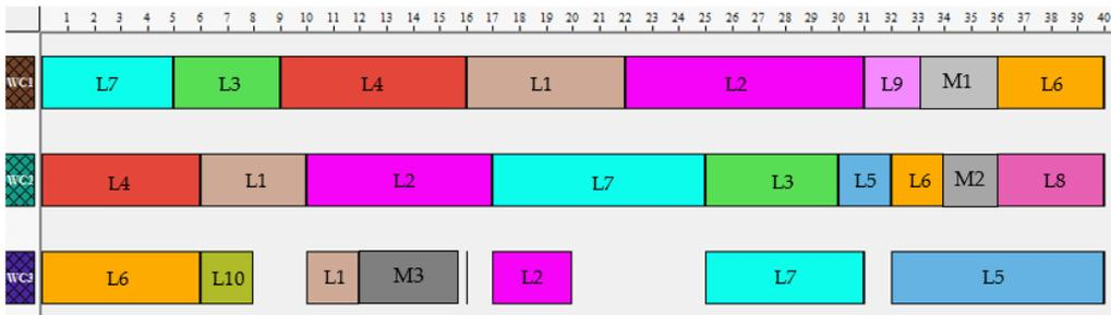
**Figure 15.** Gantt chart about the best solution found for scenario 1 (about the minimization of the internal performance measure, makespan, C<sub>max</sub>) (adapted from, (Varela, et al., 2022b))
