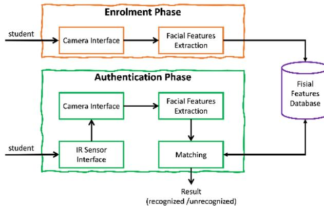
**Figure 1.** The comprehensive design model for the system of interest
