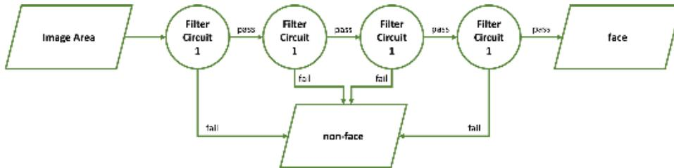
**Figure 7.** The cascade classifier structure
