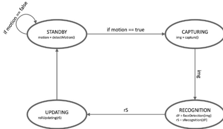
**Figure 2.** The state machine diagram for the system of interest
