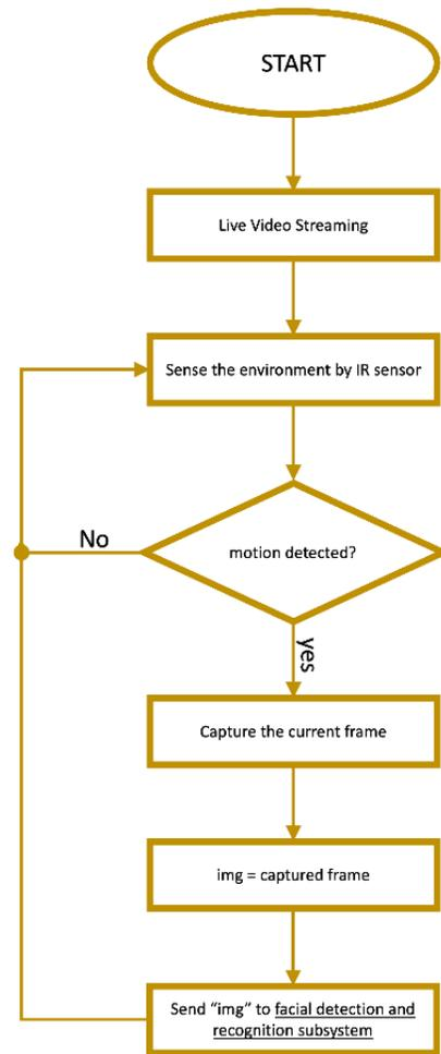
Figure 5. The functionality flowchart of the motion detection subsystem
