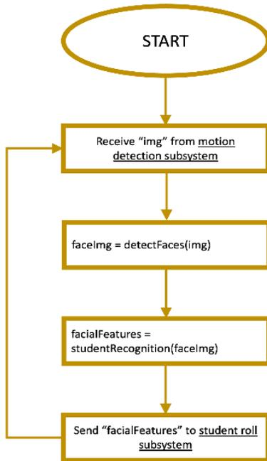
Figure 8. The functionality flowchart of the face detection and recognition subsystem
