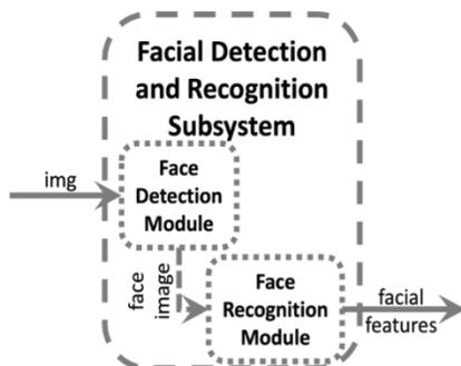
Figure 6. The detailed architecture of the facial detection and recognition subsystem
