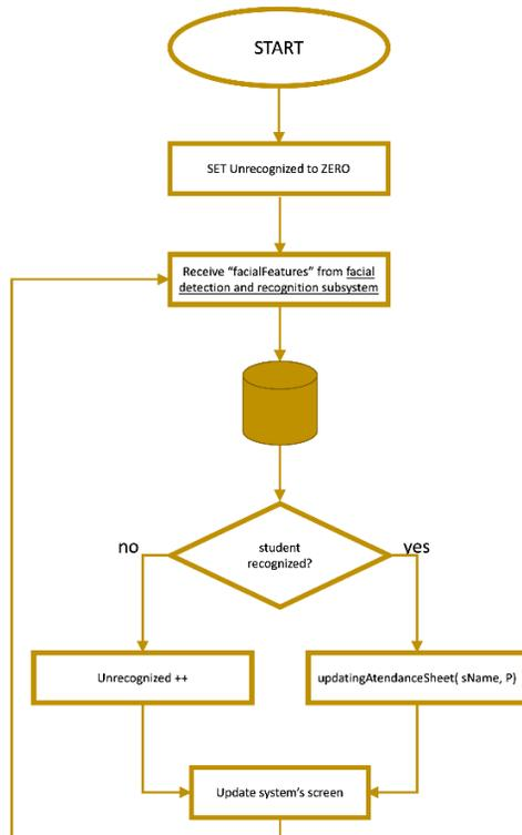
Figure 10. The functionality flowchart of the student roll subsystem
