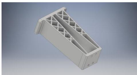
Figure 2. 3D CAD model of a car mirror holder
