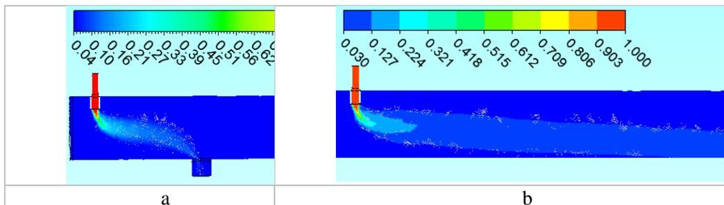
Figure 4. Fields of ethanol concentrations when fed into the first (a) and sixth (b) cylinders
