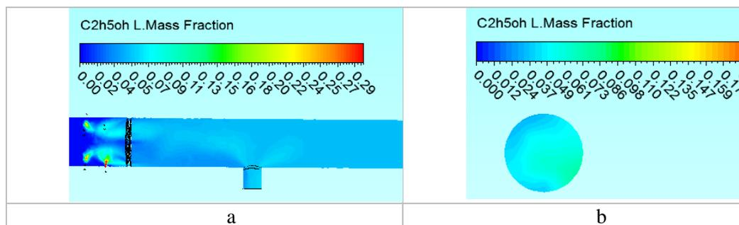
**Figure 8.** Ethanol concentrations field in the inlet header a) and in pipe nipple b) mixture supply to the first cylinder
