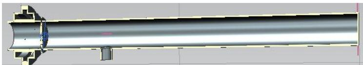
**Figure 7.** A model of a device for mixing ethanol with air assembled with an inlet header.
