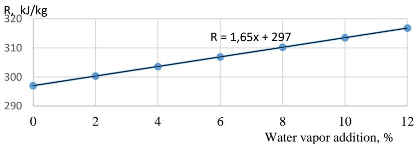
**Figure 2.** The influence of the water vapor proportion increase in combustion products on the gas constant
