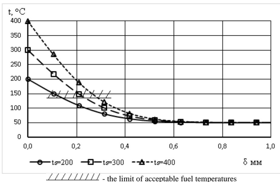
Figure 11. Distribution of fuel temperature in the channel depending on the wall temperature of the nozzle at a crankshaft speed of the D-240 diesel equal to 2200 rpm
