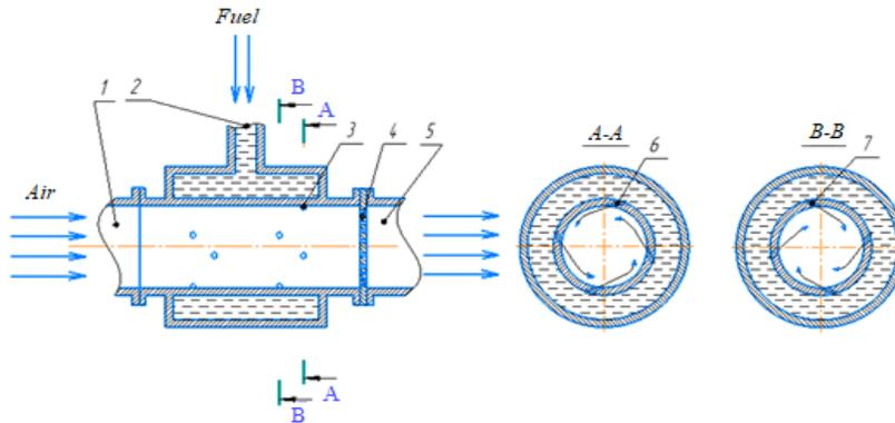
**Figure 6.** Mixing device diagram
