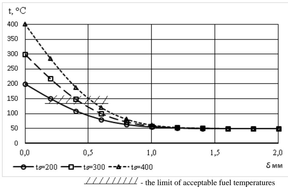
**Figure 10.** Distribution of fuel temperature in the channel depending on the wall temperature of the nozzle at a crankshaft speed of the D-240 diesel equal to 600 rpm
