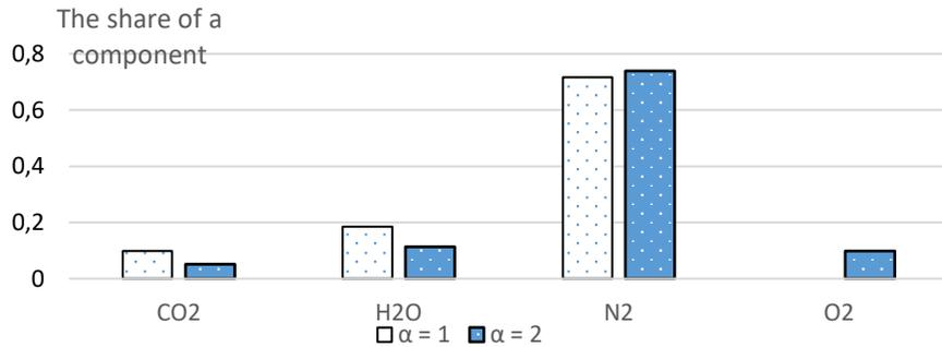
**Figure 1.** The share of the components of hydrocarbon fuel combustion products depending on the excess air ratio
