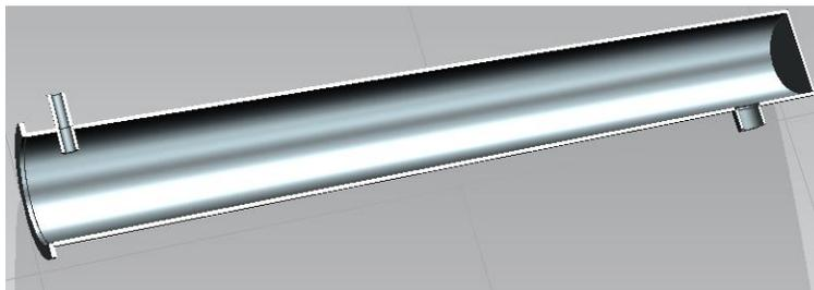
Figure 3. Inlet header with a mixture supply pipe nipple to the 6<sup>th</sup> cylinder
