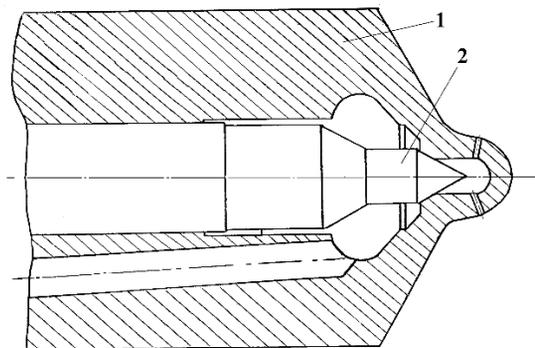
**Figure 9.** A typical layout of a diesel injector spray nozzle
