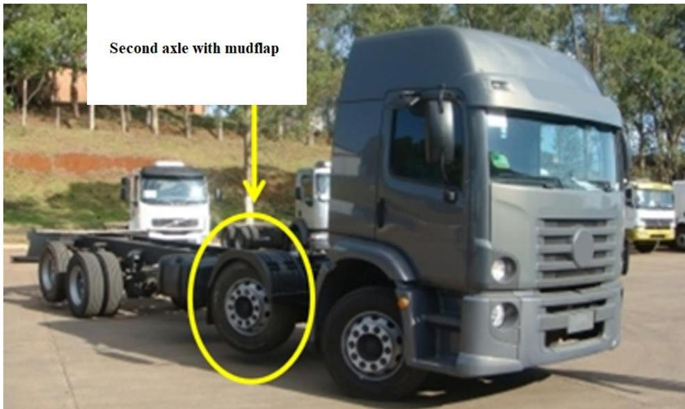
**Figure 3.** Tuck 24-ton with fender on the second steered axle implemented
