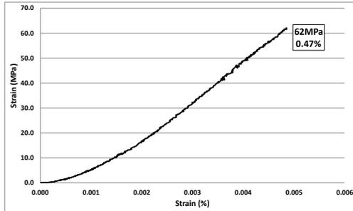
**Figure 12.** Example of stress – strain flexural diagram
