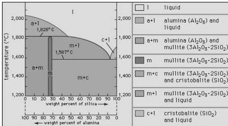
**Figure 1.** Phase diagram of the alumina-silica system related to the ceramic vitrification (Encyclopædia Britannica, Inc.)
