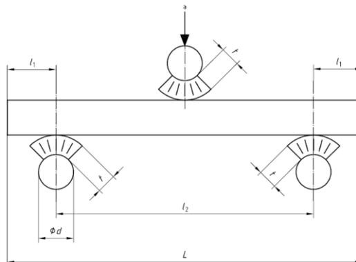
**Figure 9.** Application of loads to test specimen
