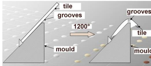
Figure 4. Bending process
