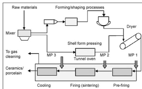
**Figure 2.** Example of process flow chart of ceramic production (by Sigma Hellas)
