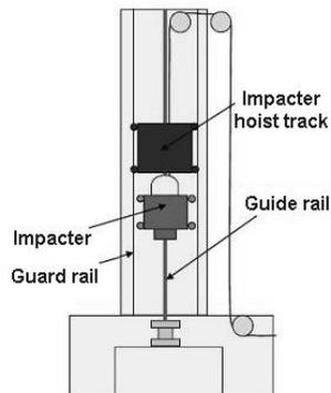
**Figure 13.** Drop-weight test equipment
