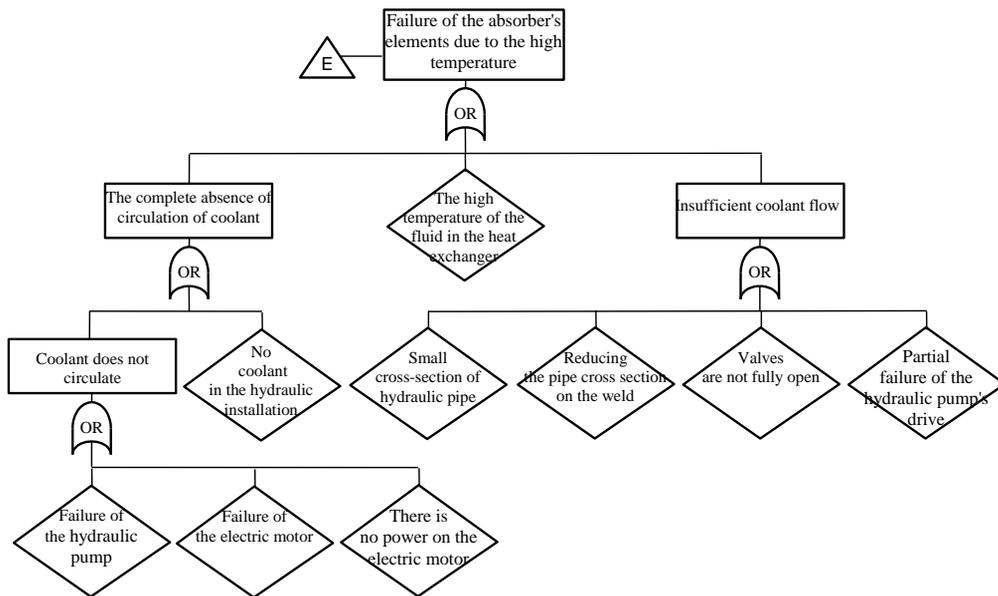
**Figure 6.** Sub failure tree for the peak event "Failure of the absorber's elements due to the high temperature"
