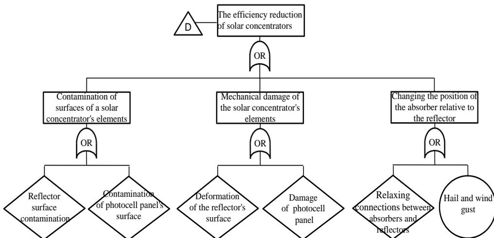
**Figure 5.** An independent sub fault tree for the peak event "Reduction of the solar concentrator's efficiency"
