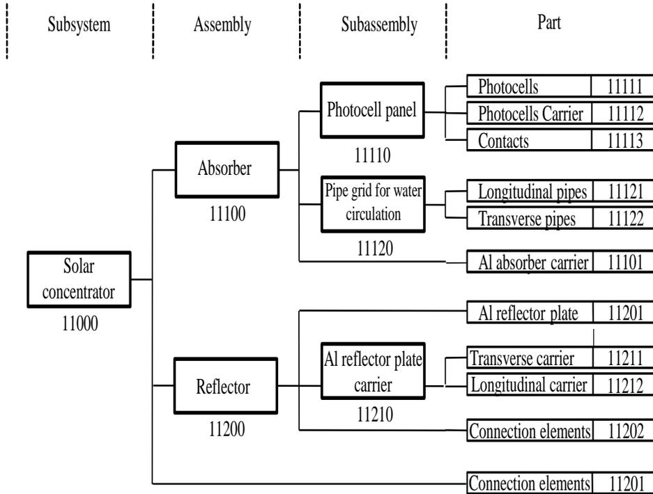
Figure 3. Scheme of dismembering of the solar concentrator
