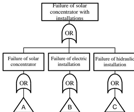
Figure 2. The parent fault tree for the peak event "Failure of the solar concentrator with installation"
