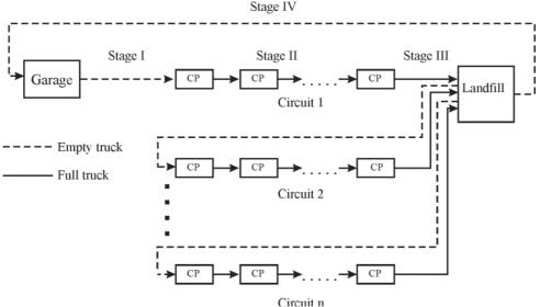
Figure 1. Stages of waste collection and transport process
