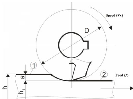
Figure 4. A basic milling process (Nedic and Lazic, 2007)
