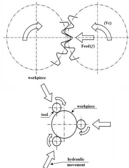
**Figure 2.** Parameters influencing the gear rolling
