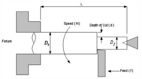
Figure 3. A basic turning process (Al-Aomar and Al-Okaily, 2006)
