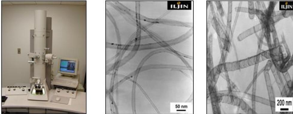
**Figure 1.** TEM apparatus and images
