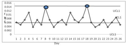
Figure 2. P (fraction nonconforming) chart
