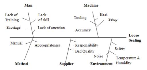
Figure 8. Cause-effect diagram for loose sealing
