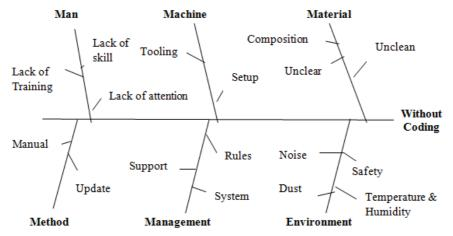
Figure 5. Cause-effect diagram for without coding
