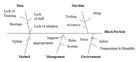
Figure 6. Cause-effect diagrams for black particle
