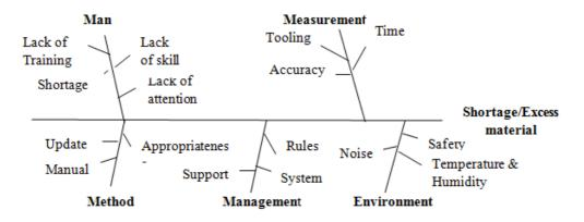
Figure 7. Cause-effect diagram for shortage/excess material
