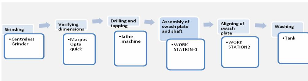
Figure 2: Line layout of investigated Process
