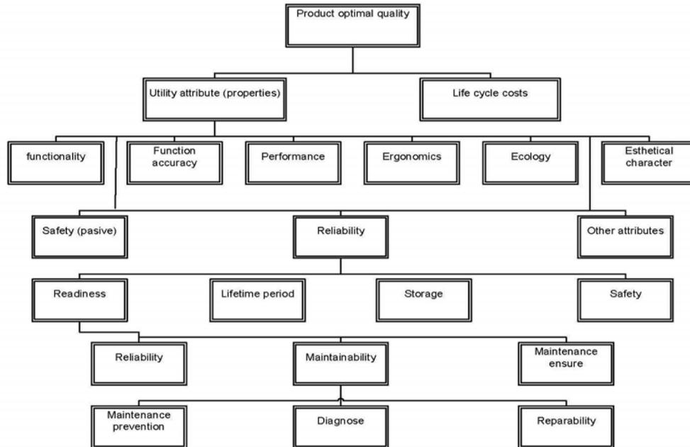
Figure 2 Criteria for evaluation of machine tool of quality and reliability
