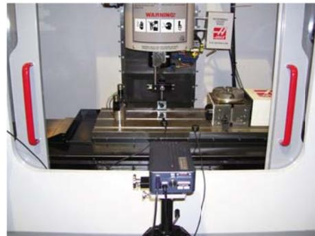
Figure. 3 Measurement using Laser interferometer
