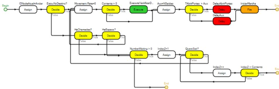
**Figure 2.** Process responsible for deciding an elevator stop
