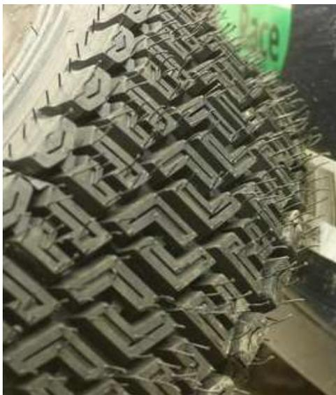
**Figure 13.** Tire vents [Courtesy of Doug Chase]
