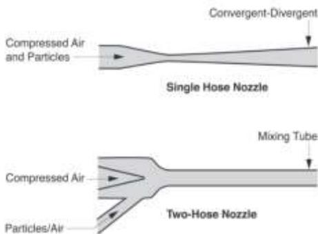
**Figure 19.** The two possible systems for blasting cleaning technologies (Foster, 2005)
