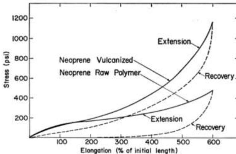
**Figure 10.** Effect of vulcanization of a neoprene synthetic elastomer with no fillers (J. Campbell, 1963)
