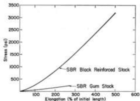
**Figure 6.** Vulcanized SBR with 30% carbon black compared with natural SBR (Campbell, 1963)
