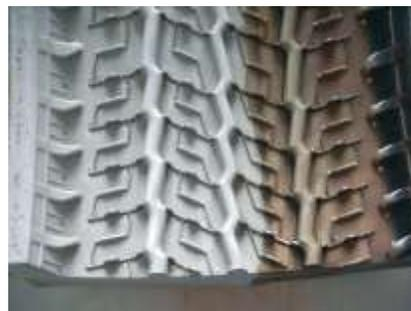
**Figure 17.** Tire mould partially cleaned. The brown part is still dirty [Courtesy of Clean Lasersysteme GmbH]
