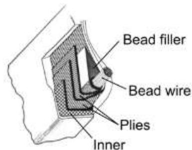
**Figure 3.** Detail of a typical bead (Gough, 1981)
