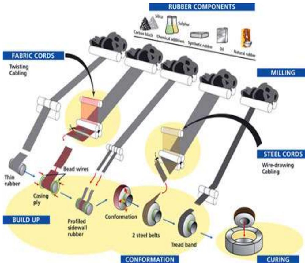
**Figure 7.** Schematic representation of the production process of a tire [Courtesy of WBCSD]
