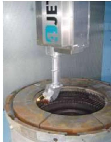
**Figure 21.** Automatic laser cleaning
