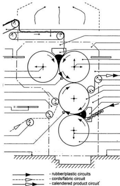
**Figure 9.** Calendaring of plies [Courtesy of HSE]
