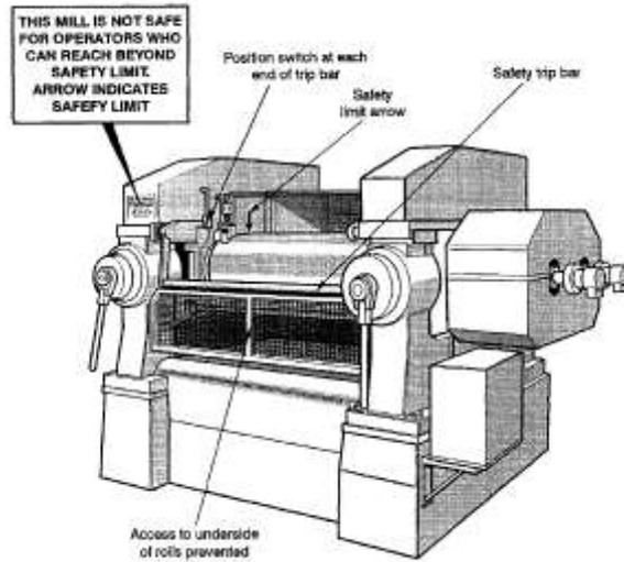
**Figure 8.** The open mixer, in which the compound, which came out from the Banbury mixer, is inserted [Courtesy of HSE]
