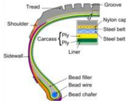
**Figure 2.** Schematic structure of a radial tire [Courtesy of Wikimedia Commons]
