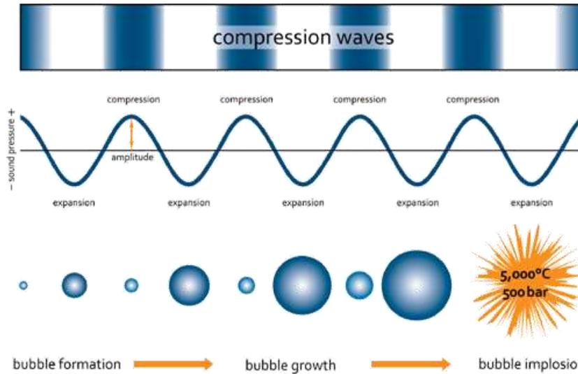
**Figure 22.** Operating principle of ultrasonic cavitation [Courtesy of Ultrawaves GmbH]
