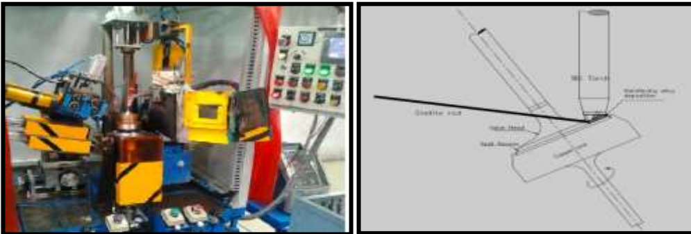
Figure 6. TIG welding machine and partial schematic drawing of seat hardfacing process
