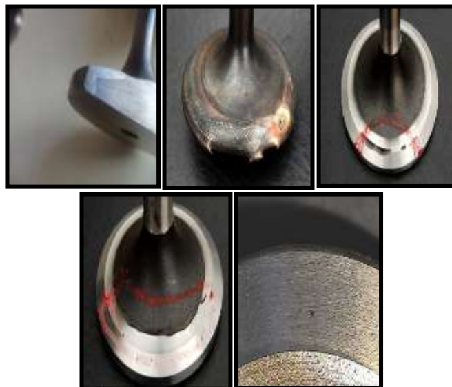
Figure 5. Photograph of I.C. Engine Valves defects
