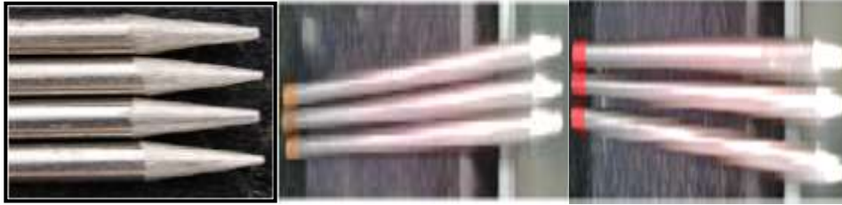
Figure 10. 2% Thoriated tungsten and 1.5% Lanthanum tungsten electrodes and proposed tip preparation
