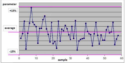
Figure 14. Control chart regarding the flexural resistance of bended tiles
