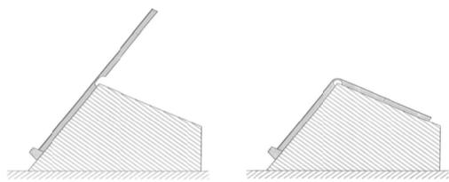
Figure 1. Bending process for a tile
