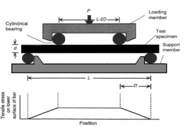
Figure 5. Application of loads with 3-point and 4-point flexural test
