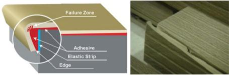
Figure 6. Tile failure
