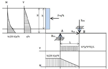
Figure 12. Evaluation scheme of loads (F), reaction forces (R), shears (V) and bending moments (M)
