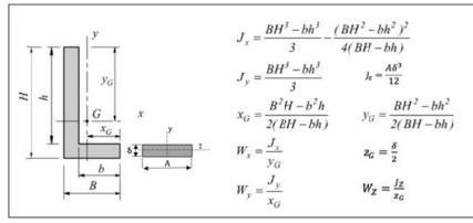
Figure 11. Standard formula for an "L" shaped beam
