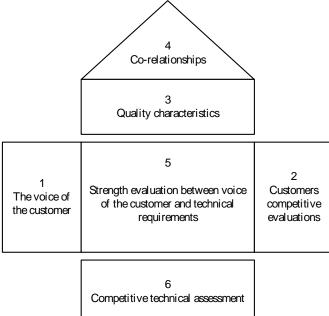
Picture 1. Components of horizontal and vertical matrix part
