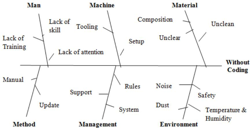
Figure 5. Cause-effect diagram for without coding
