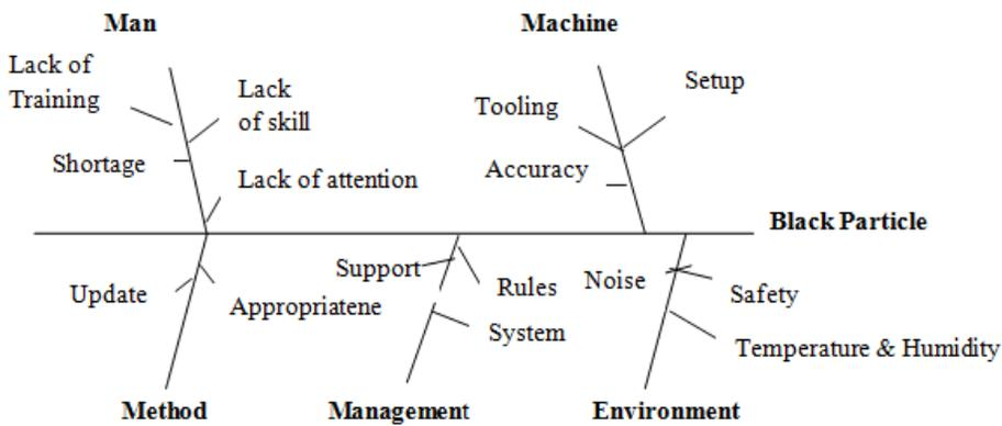
Figure 6. Cause-effect diagrams for black particle
