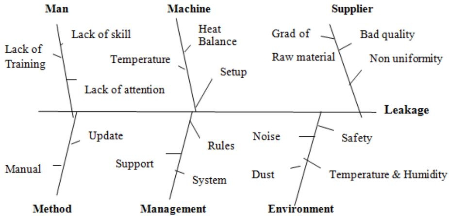
Figure 4. Cause-effect diagrams for leakage
