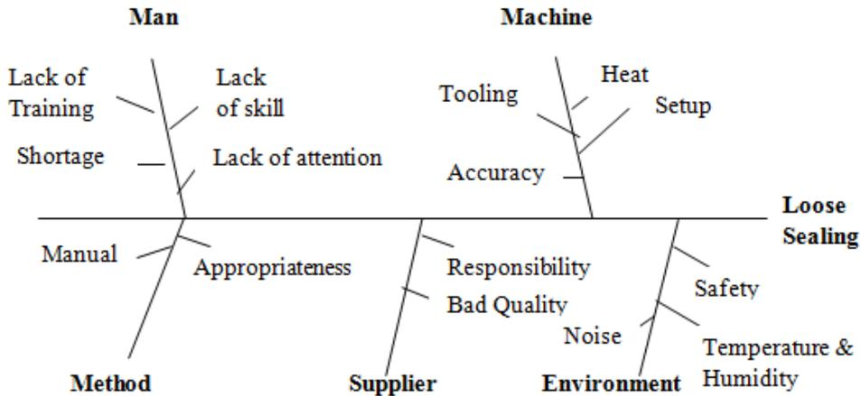
Figure 8. Cause-effect diagram for loose sealing
