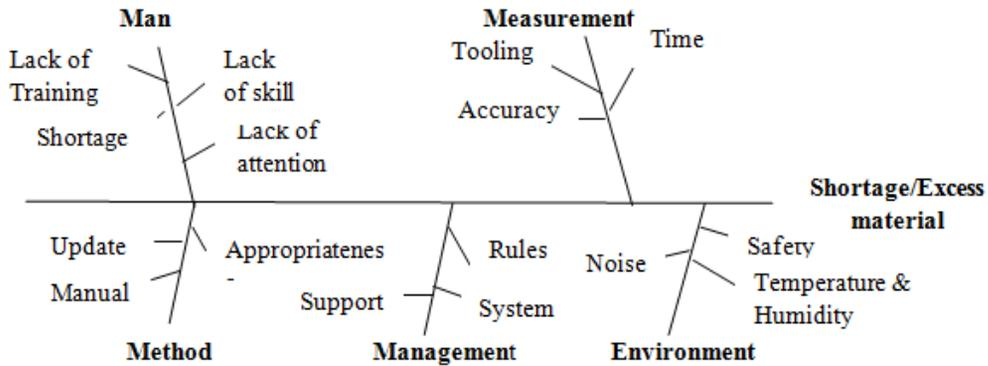
Figure 7. Cause-effect diagram for shortage/excess material
