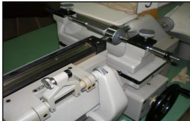
Fig.10 The vertical control of the plate gauge.
