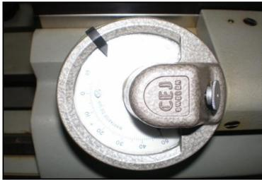
Fig.8 The adjustment of the force of the measuring instrument.
