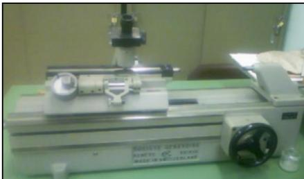
Fig.1 Industrial Optic Accuracy Micrometer  $0,01 \mu\text{m}$
