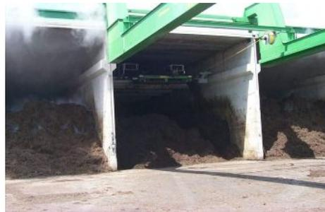
*Figure 6. Facility for composting*
