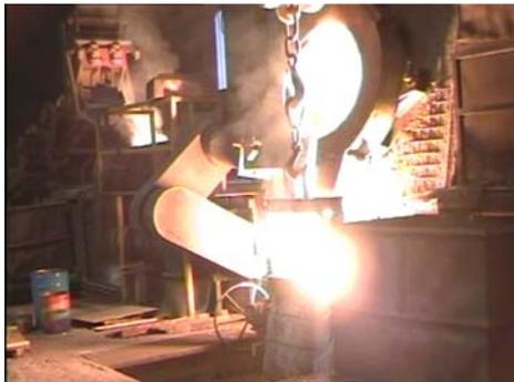
*Figure 2 - Melting in induction furnace*
