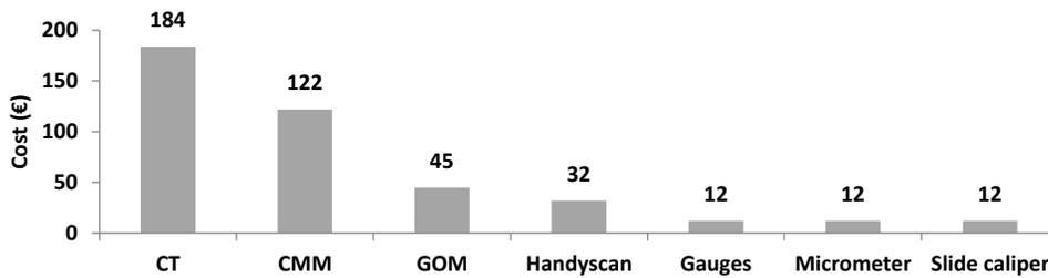
Figure 5. Car mirror holder measurement cost chart
