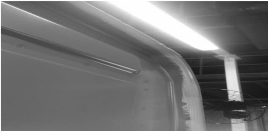
**Figure 1.** Viscous mass applied to the vehicle body
