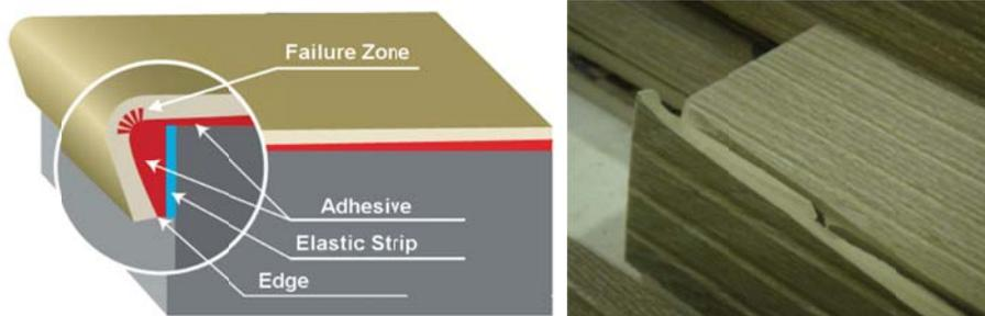
**Figure 6.** Tile failure
