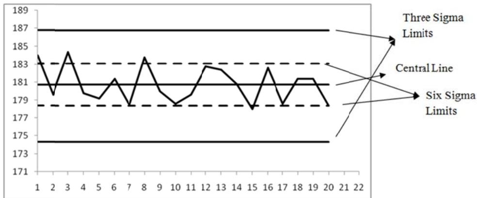
**Figure 2.** Six Sigma-based and traditional X-bar control charts
